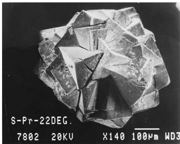
Figure 7 Interpenetrating multiple praseodymium heptamolybdate crystals leading to complex twinning and giving the appearance of spherulitic formation.
